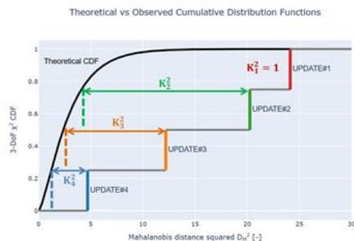
Figure 13 – K-Interval coefficient method
