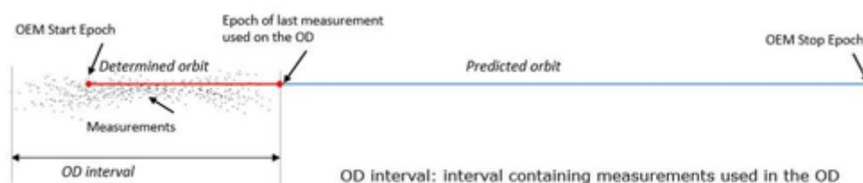
Figure 20 – Determined orbit and predicted orbit
