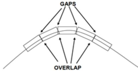
Figure 10 – Tube sections for non-linear relative motion. Gaps and overlaps are visible (from [REF. 4])
